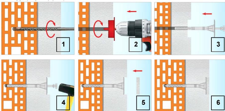
1) Drill the hole perpendicular to the substrate surface. Clean the drill hole.
