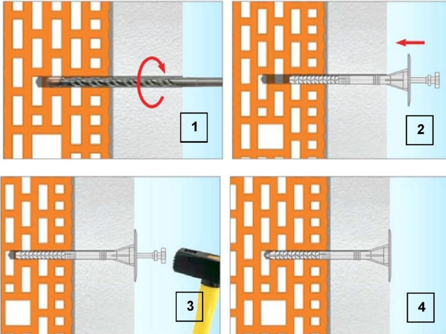
1) Drill the hole perpendicular to the substrate surface. Clean the drill hole.
