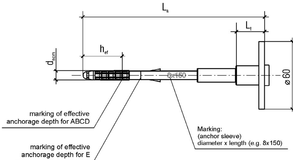
**Screw with an additional coating of the screw head**
