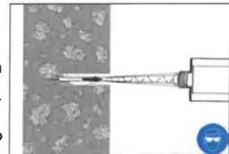
6. Insert the mixer nozzle (resin stopper / extension tube if applicable) to the bottom of the hole. Begin to extrude the resin and slowly withdraw the mixer nozzle from the hole ensuring that there are no air voids as the mixer nozzle is withdrawn. Fill the hole to approximately 1/2 to 3/4 full and remove the mixer nozzle completely.
