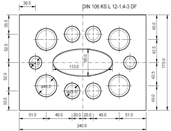
Hollow sand lime brick KSL 12-1,4-3DF according to EN 771-2
