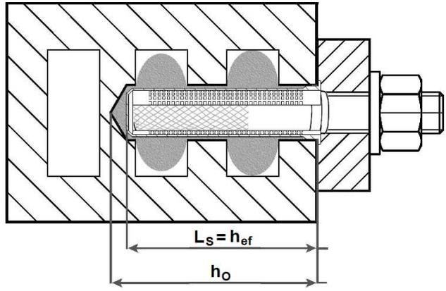
**Installation in solid brick masonry**
