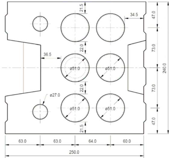
Hollow sand lime brick KSL 12-1,4-8DF according to EN 771-2
