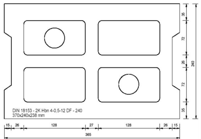
Concrete masonry unit Hbn 4-12DF
