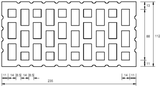
Hollow clay brick HLz 12-1,0-2DF according to EN 771-1
