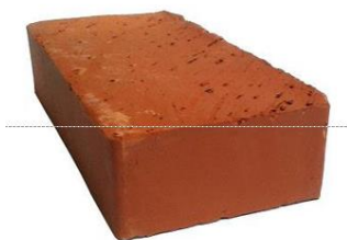
Solid clay brick Mz-NF according to EN 771-1 length/width/height = 240 mm / 115 mm / 71 mm f_b \geq 20 \text{ N/mm}^2 / \rho \geq 1,9 \text{ kg/dm}^3
