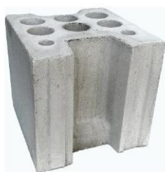
Perforated calcium silicate brick KSL-R-12-1,2-16DF according to EN 771-2 length/width/height = 239 mm / 248 mm / 239 mm f_b \geq 15 \text{ N/mm}^2 / \rho \geq 1,3 \text{ kg/dm}^3
