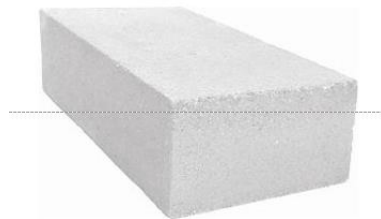
Solid calcium silicate brick KSV-NF according to EN 771-2 length/width/height = 240 mm / 115 mm / 71 mm f_b \geq 25 \text{ N/mm}^2 / \rho \geq 1,8 \text{ kg/dm}^3
